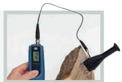
APPLICATION Moisture measurement perpendicular to the wood fibre direction using an M 20 electrode
